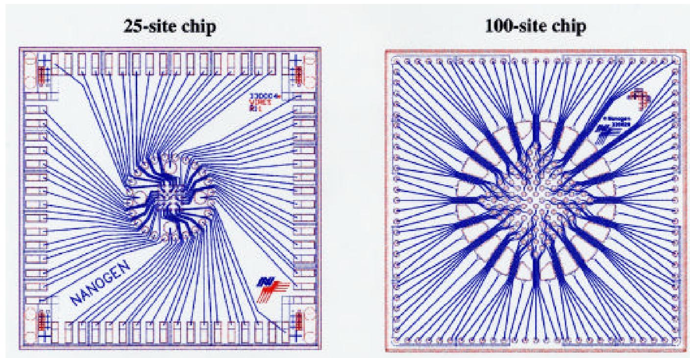
**Figure 1:** Layout for the 25-site and 100-site chips. The array (5 x 5 or 10 x 10) is in the center of the microchip. The ring pads surrounding the array are used as counter electrodes. Contact pads are on the edge of the chip, which are used for contacting with pogo pins that apply electronics to the microchip. For each of the test sites and ring pads, there is a platinum wire connecting it to its respective contact pad. There are two wires for each test site on the 25-site chips.
