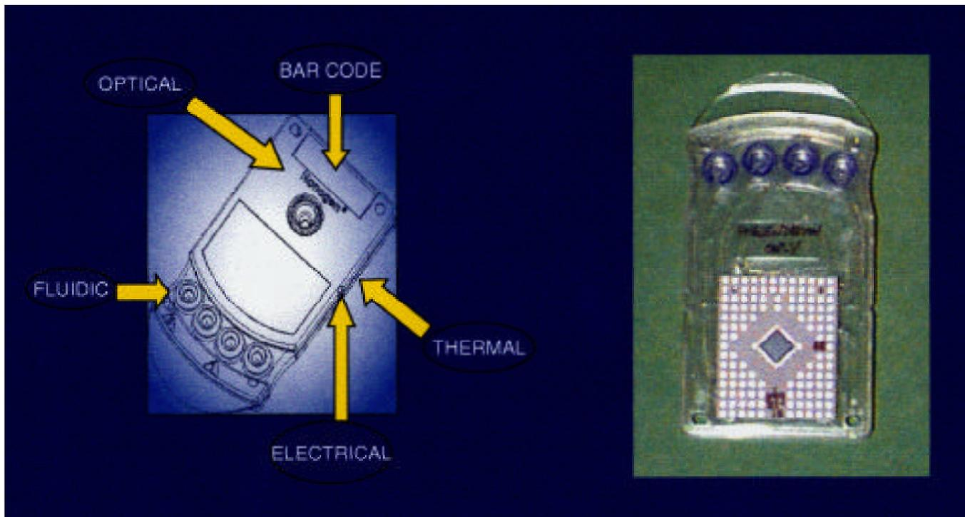
**Figure 4:** The Nanogen microchip cartridge. The cartridge contains a 100-site microchip mounted on a substrate that has contact areas for electrical pogo pins (panel on the right). A flow cell sits on top of the array and serves as a chamber for electronics, washing and optical window (panel on the left). The cartridge also contains multiple valves and interconnected channels leading to the flow cell for sample application and washing.
